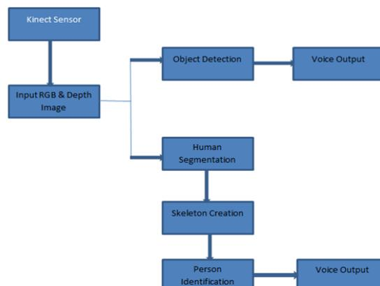
The framework is made out of 4 fundamental parts: profundity camera, object recognition, Human division and Skeleton creation. In this examination, Kinect camera is utilized as the profundity camera. The goals of the picture furnished by this camera is 640x480 with 30 outlines for each second. The viable scope of the camera is inside 0.8 meter to 4 meter, with even and vertical vision point of 57.5° and 43.5° separately.
