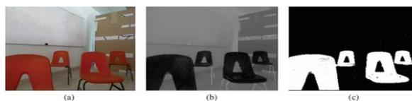
**(a) RGB color image (b) Euclidean distance from each pixel to the point of interest (the probabilistic image) (c) Initial mask.**
